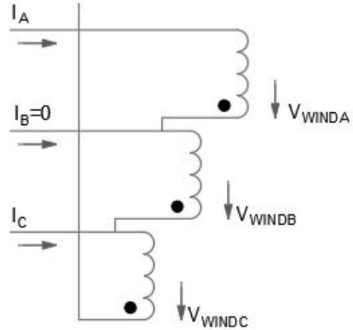
Fig. 3 High Side Delta with Loss of Phase B [2]
