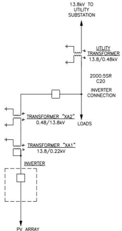
Fig. 1 Single Line Interconnection with Transformer Network to Mitigate Voltage Drop
