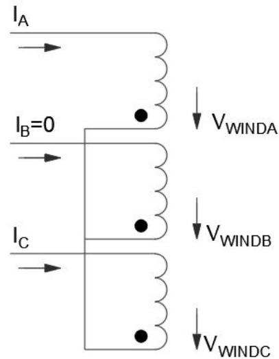
Fig. 4 High Side Wye with Loss of Phase B [2]
