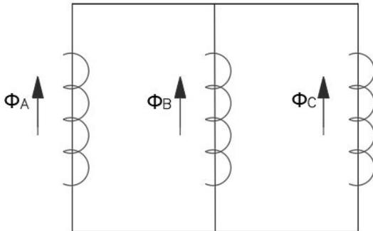
Fig. 2 Flux and Voltage in a Three-Legged Core [2]
