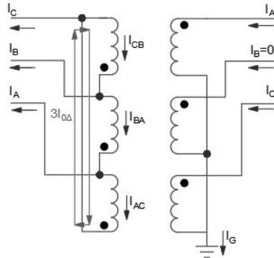
Fig. 7 Open Phase, Yg-Δ Transformer [2]
