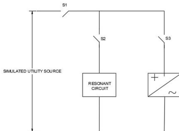
Fig. 5 Inverter Anti-Islanding Test with Balanced Load [3]
