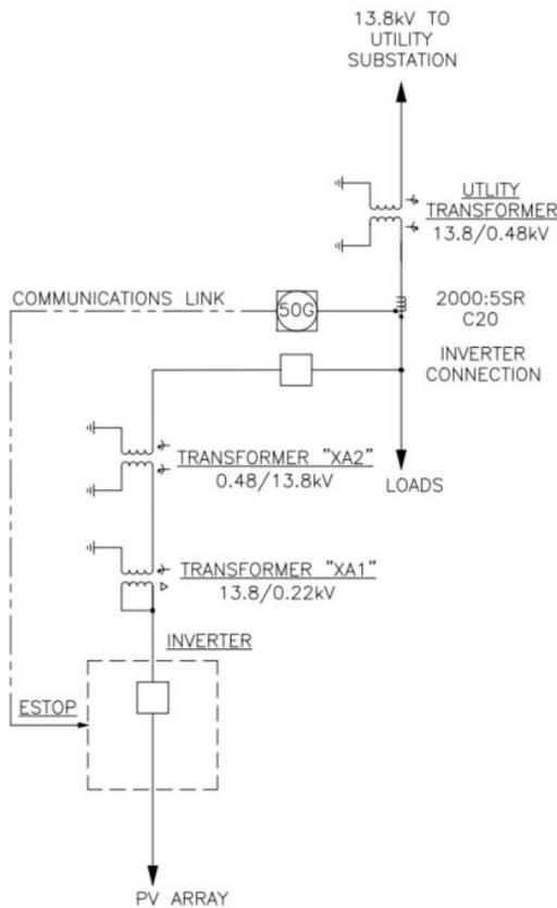
Fig. 6 System Single Line Diagram
