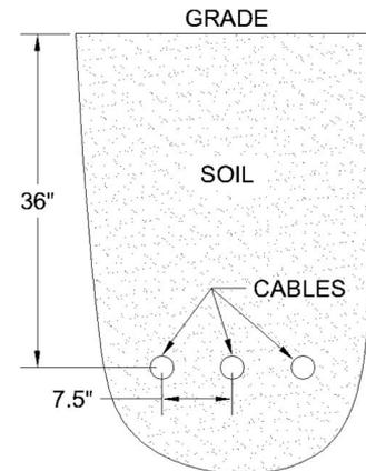
Fig. 1. Cable configuration.
