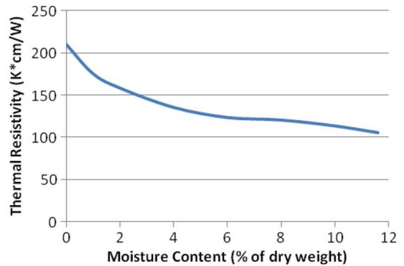
Fig. 4. Soil dry out curve.
