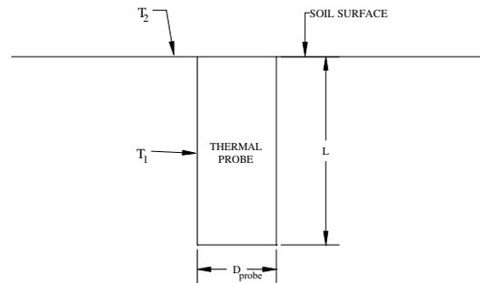
Fig. 2. Thermal probe test for non-drying heat rate.
