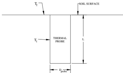
Fig. 2. Thermal probe test for non-drying heat rate.
