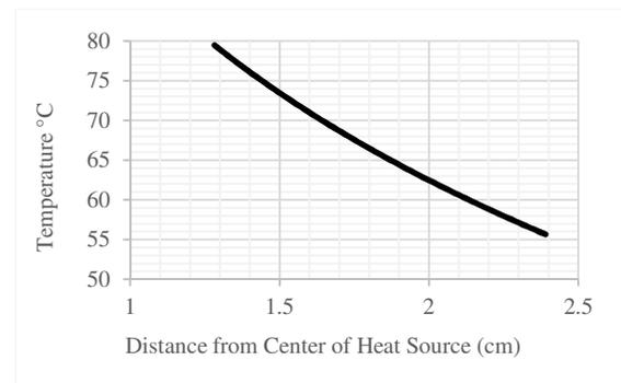
Fig. 4. Temperature from heat source surface to extent of dried area.
