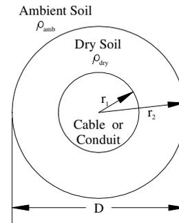
Fig. 1. Model of soil drying.
