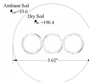
Fig. 5. Cables inside dried soil layer.
