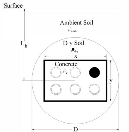
Fig. 6. Concrete duct bank enclosed in dried soil.
