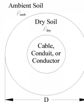
Fig. 1. Model of cable including dried soil caused by thermal instability.
