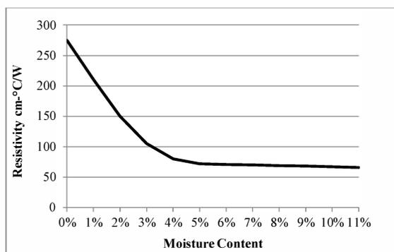
Fig. 2. Soil dry-out curve for sand.
