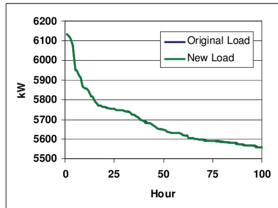
Figure 5. Feeder A - LDC Top 100 hours
