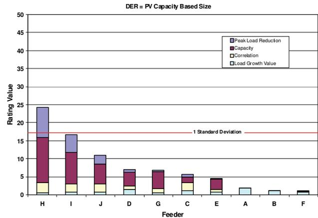
Figure 8. Case 1: Feeder Value and Ranking
