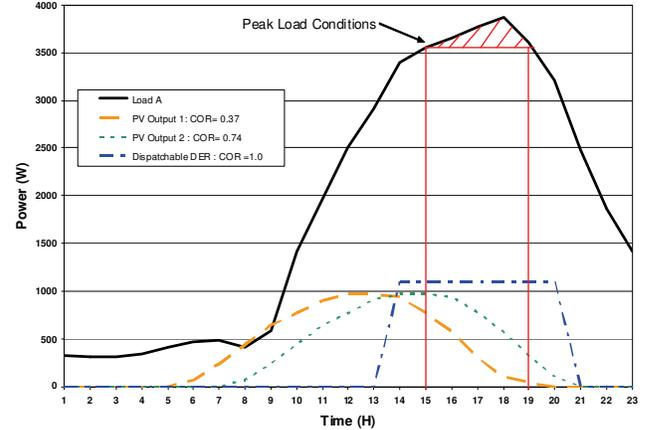
Figure 2. COR Factor with Various DER
