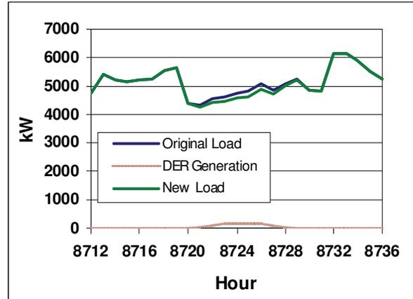
Figure 4. Feeder A – Peak Load Day with PV
