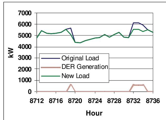
Figure 9. Feeder A – Peak Load Day with Dispatchable DER
