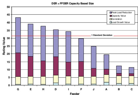
Figure 13. Case 6: Feeder Value and Ranking
