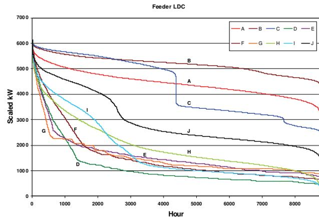
Figure 3 Normalized LDCs for All Feeders
