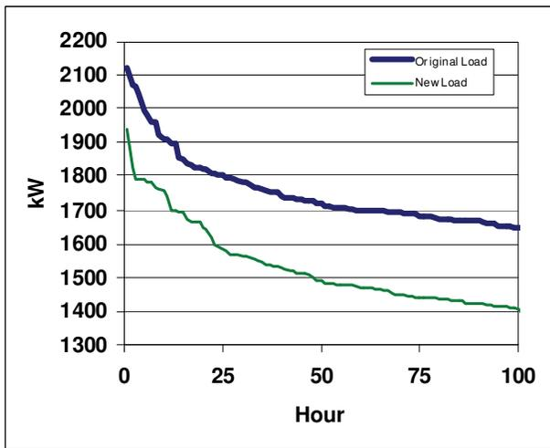
Figure 7. Feeder H – LDC Top 100 Hours
