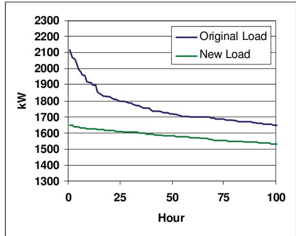
Figure 12. Feeder A – LDC with Dispatchable DER
