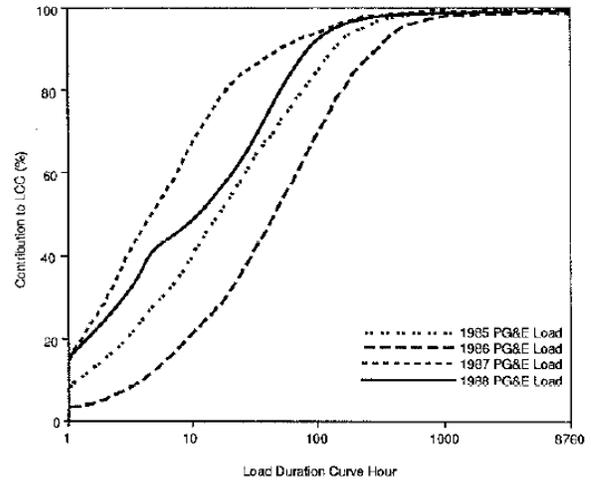
Figure 1. LCC as a Function of LDC Hour<sup>[9]</sup>
