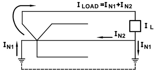
Figure 7(a) Neutral current flowing in neutral and ground
