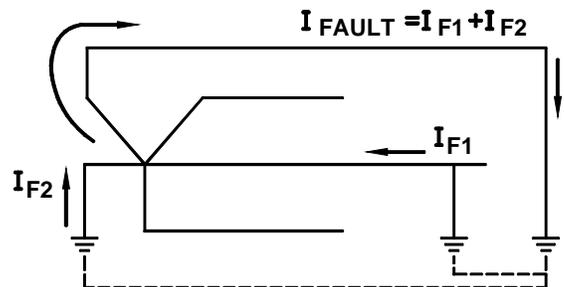
Figure 7(b) Ground fault current flowing in the neutral and ground
