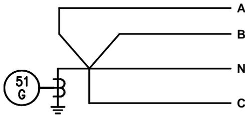
Figure 6(a) Current transformer in ground
