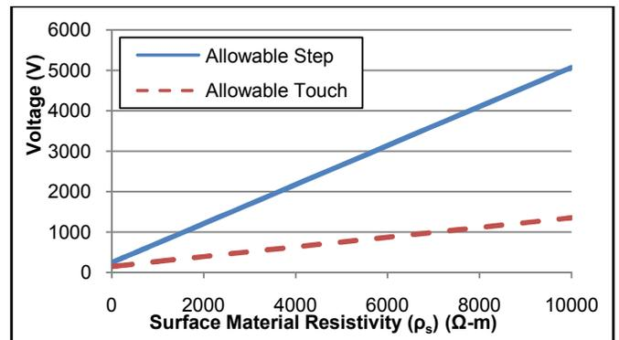
Figure 1 Effects of surface material resistivity on allowable touch and step voltages
