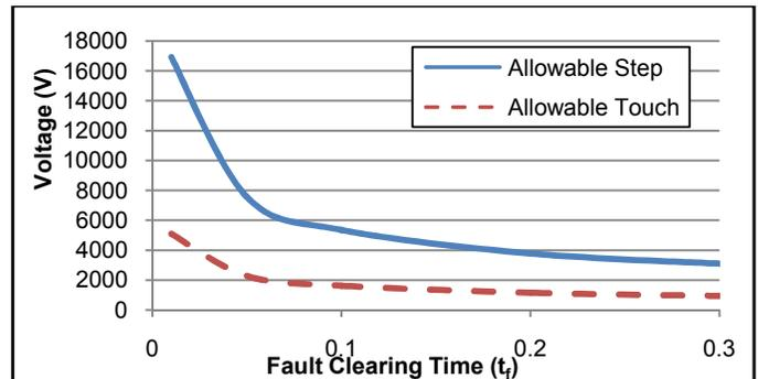
**Figure 5** The effect of fault clearing time on allowable step and touch voltages
