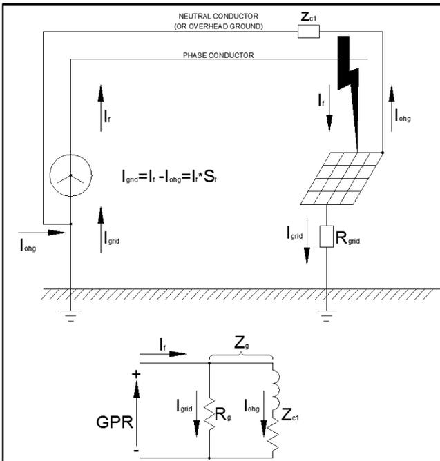
**Figure 3** The grid current is only a fraction of the fault current when a shield or neutral is present. [1:9]
