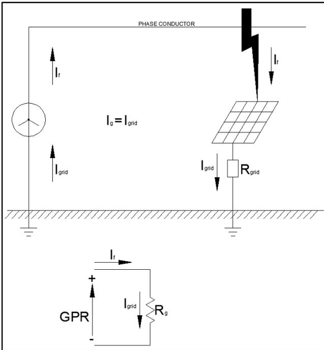
**Figure 2** The grid current equals the fault current when no shields or neutrals are present. [1:9]
