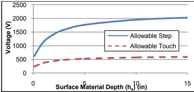
**Figure 4** Effects of surface material depth on allowable step and touch voltages
