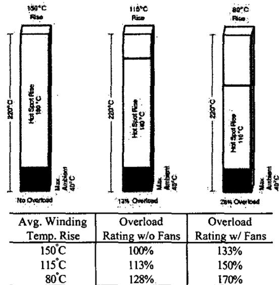
Figure 2. Overloading Capability of Transformer with 220°C Insulation System
