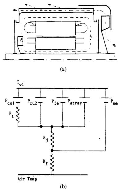
Fig. 3. Totally enclosed fan-cooled squirrel-cage motor. (a) Air flow. (b) Thermal network.
