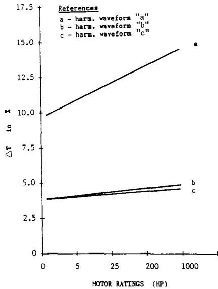
Fig. 6. Temperature increase on totally enclosed fan-cooled induction motor.
