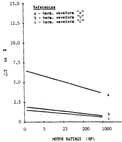
Fig. 5. Temperature increase on drip-proof radially cooled induction motor.
