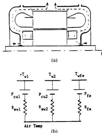
Fig. 2. Drip-proof radially cooled squirrel-cage motor. (a) Air flow. (b) Thermal network.
