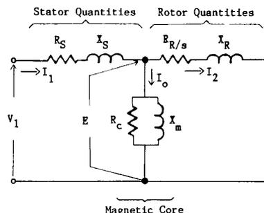
Fig. 1. Equivalent circuit of induction motor.
