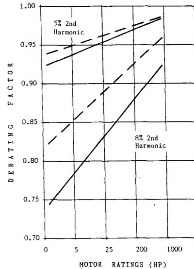
Fig. 7. Derating factors due to harmonic voltage distortion. Dotted lines: drip-proof radially cooled motor. Solid line: totally enclosed fan-cooled motor.
