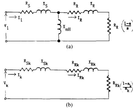
Fig. 4. Equivalent circuit for induction motor with nonsinusoidal excitation. (a) Fundamental. (b)  $k_h$  harmonic.
