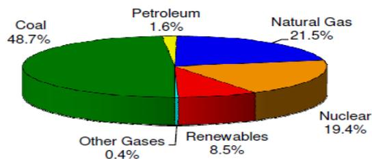
Fig. 1 Electric Energy Production in the USA by Fuel Type.
