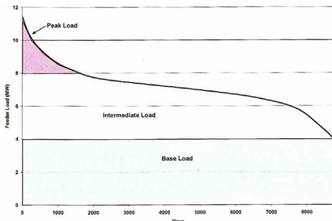
Fig. 6 Typical Annual Load Duration Curve.
