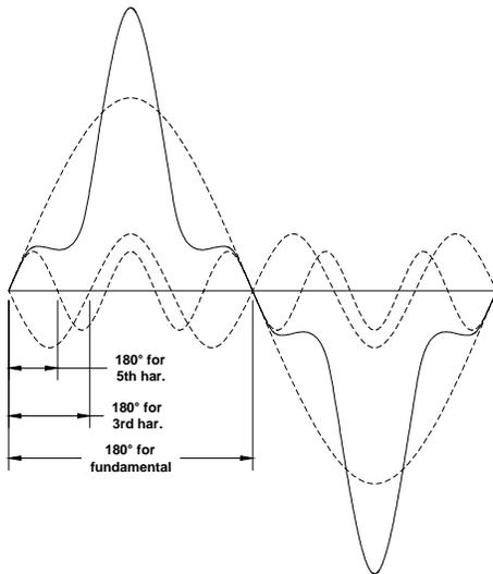
Fig. 2 – Magnetizing Current
