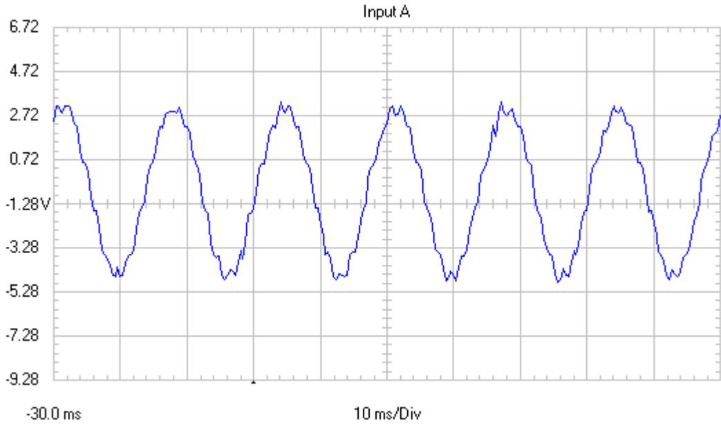
VSD1 - 12 Pulse 520 kVA Drive Std Current Waveform
