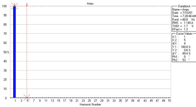
Fig. 11 – Harmonic Current Profile w/o drives
