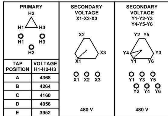
Fig. 9 – Closed Polygon Transformer
