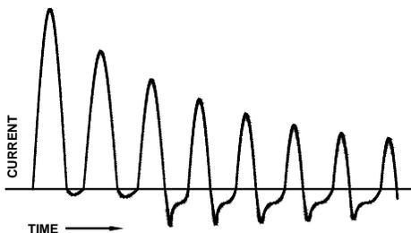
Fig 3 – Transformer Inrush Current
