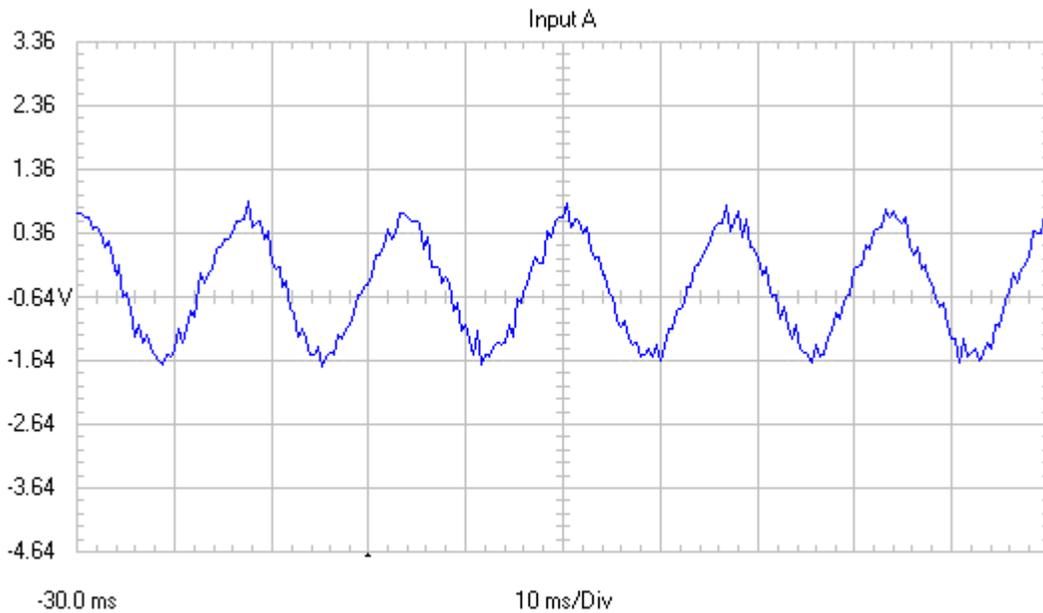
ESP Building Power Source - Quasi 24 Pulse System - A Phase Current
