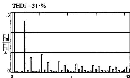
Fig. 2. Current harmonics of one phase shown in Fig. 1.
