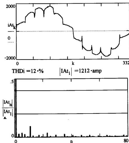
Fig. 21. Phase "A" current summation and harmonic spectrum of Lifts #1 and #2 with nearly equal firing angles.
