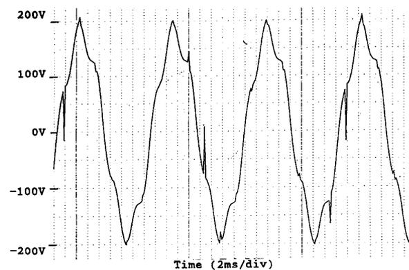
Fig. 3. Voltage waveform showing the extra zero crossings caused by a six-pulse converter.
