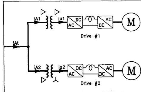
Fig. 6. Two constant current, six-pulse motor drives connected through step-down transformers to achieve harmonic cancellation.
