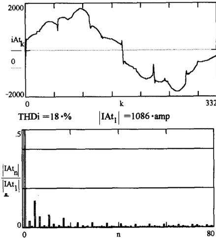
Fig. 22. Typical operating conditions: Phase "A" current summation and harmonic spectrum of Lifts #1 and #2 with uncontrolled firing angles.
