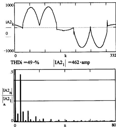
Fig. 19. Lift #1 phase "A" time domain current waveform and harmonic spectrum.
