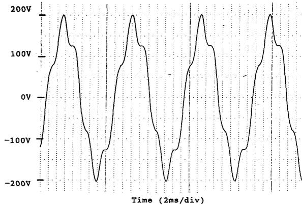
Fig. 4. Twenty-five kilovolt bus PT's showing the voltage amplification from parallel resonance when capacitor banks are connected to the system.
