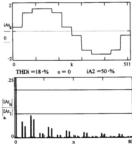
Fig. 14. With  $\alpha = 0$ ,  $iA2$  is adjusted to 50% of  $iA1$ .
