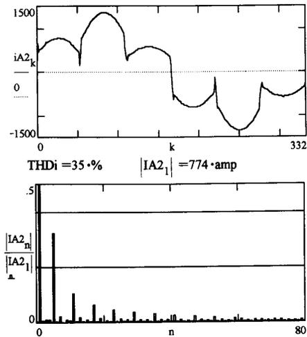
Fig. 20. Lift #2 phase "A" time domain current waveform and harmonic spectrum.
