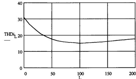
Fig. 16. THDi versus relative loading between drives from 0 to 200% at  $\alpha = 0$ .
