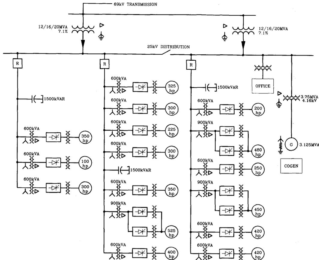
Fig. 17. One-line diagram of a distributed set of VFD loads used in an oil field.
