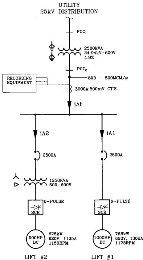
Fig. 18. One-line diagram of independent six-pulse ac/dc converter motor drives used for two detachable-quad ski lifts.
