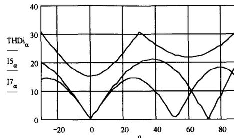
Fig. 13. THDi versus  $\alpha$  for equal drive currents.
