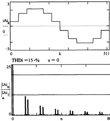
Fig. 9. Twelve-pulse current summation and harmonic magnitude spectrum for  $\alpha = 0$  and equal drive current amplitudes.
