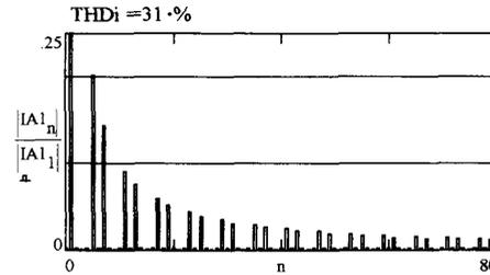
Fig. 8. Harmonic magnitude spectrum for all six-pulse converter waveforms shown in Fig. 7.
