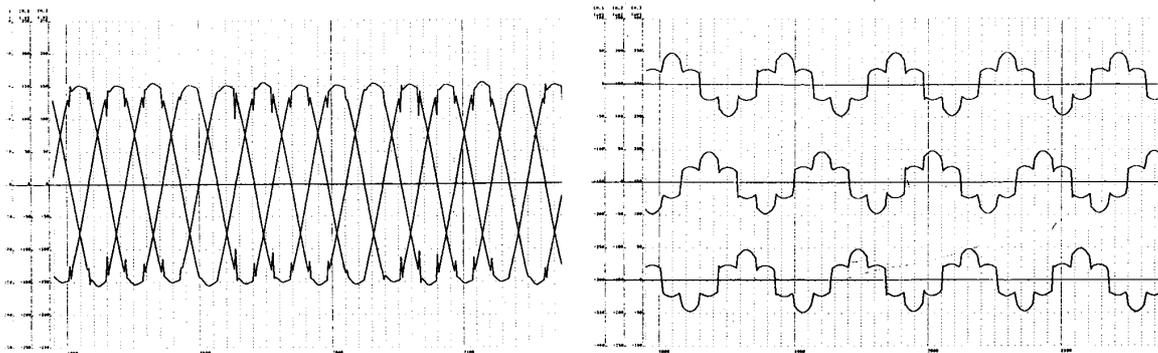
Fig. 1. Time-domain voltage and current waveforms of a 3000-hp, six-pulse, load commutated inverter drive as viewed from the source.
