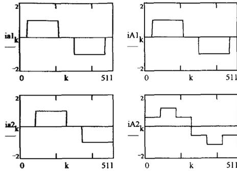
Fig. 7. Time domain current waveforms of the dual converter drive connections shown in Fig. 6.
