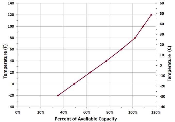
Figure 5. % of Battery Capacity vs. Ambient Temperature [12]
