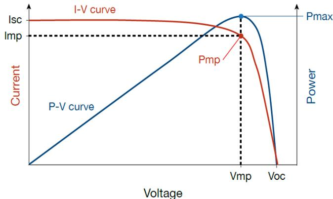
Figure 2. Normal IV curve and PV Curve from a Single Cell [10]
