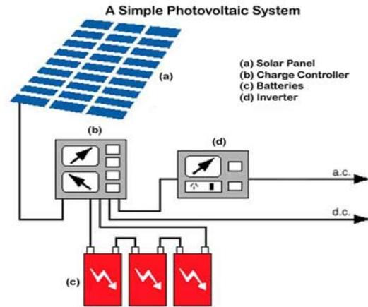
Figure 3. Schematic of a Stand-Alone PV System [11]
