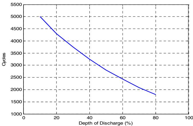
Figure 4. Depth of Discharge (%) vs. Number of Cycles for Typical Deep-Cycle Lead-Acid Battery [3]
