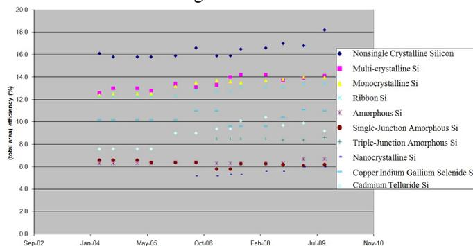
Figure 1. Best Average Commercial Module Efficiency by Technology [2]
