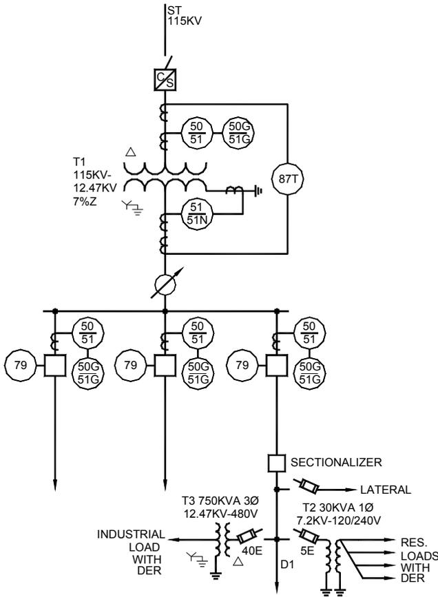
Figure 1. Typical Power Distribution System Including Protection
