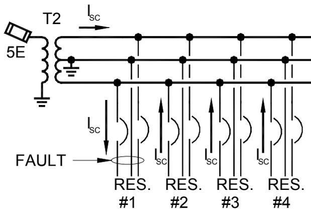
Figure 2. Fault condition with residential DER
