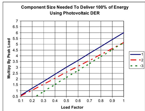
Figure 4. Component size needed to allow delivery of 100% of PV energy
