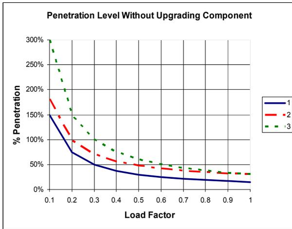
Figure 5. Allowable penetration levels without component upgrade for PV DER
