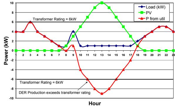
Figure 7. Good DER Production and Load Coincidence
