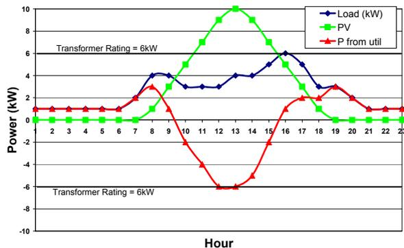
Figure 6. Case A. Good DER Production and Load Coincidence
