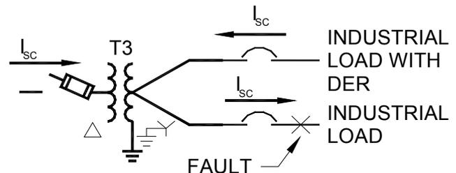
Figure 3. Fault with DER on customer side of transformer
