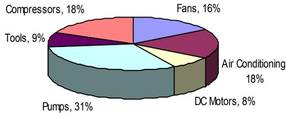
Figure 5: How motors are used.
