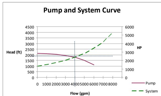
Figure 7: Pump operating curve after reduction in pump speed.
