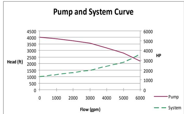
Figure 6: Typical pump and system curve.
