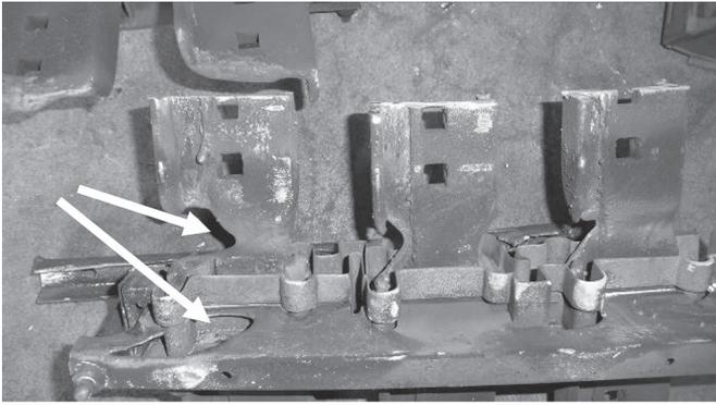
Fig. 2. Arc damage from outside phases to enclosure supports for a three-phase fault.
