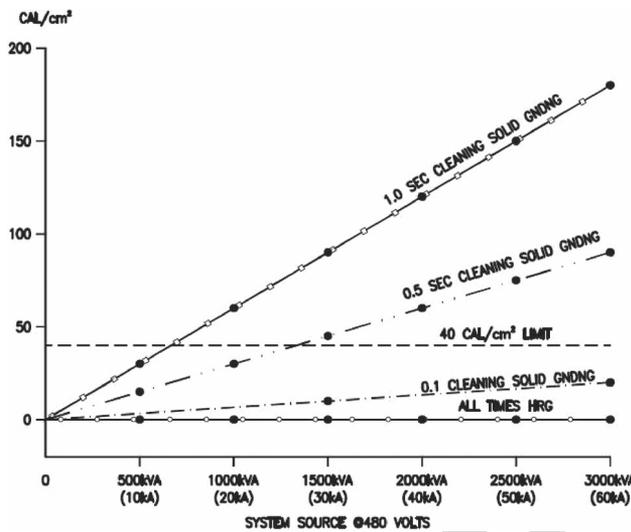
Fig. 3. Incident energy levels for solid versus high resistance grounding.
