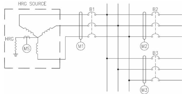
Fig. 5. Ground fault sensing.
