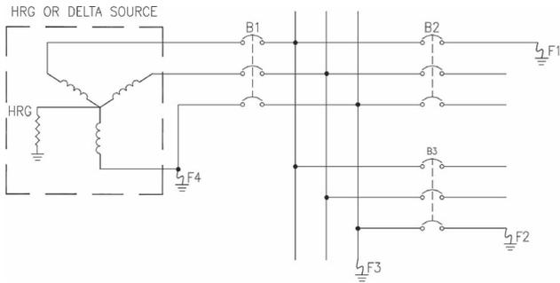
Fig. 4. Single-pole tripping.
