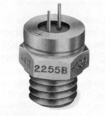
**Figure 6: Shock Sensor**
