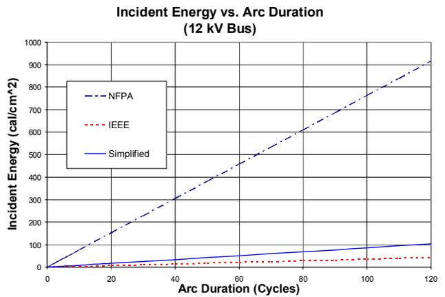
Fig. 12 Comparison of Incident Energy Calculations
