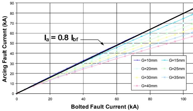
Fig. 4 Sensitivity to Gap between Conductors: 600V and Below
