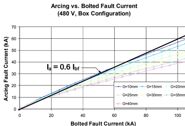
Fig. 1 Sensitivity to Gap between Conductors: 480V and Below
