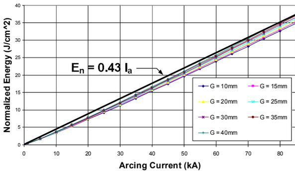
Fig. 6 Sensitivity to Gap between Conductors: 600V and Below
