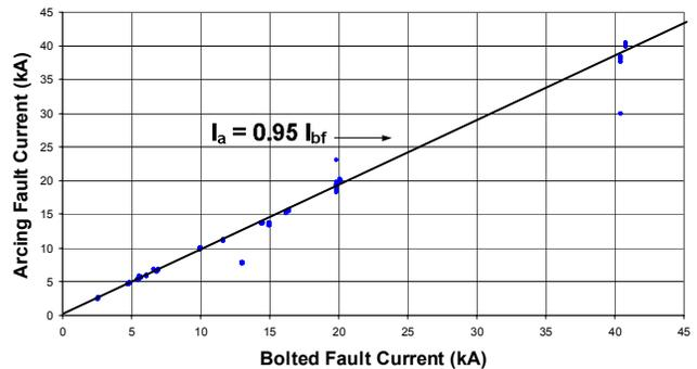
Fig. 8 Scatter-Plot of IEEE 1584 Medium Voltage Test Data: Over 1kV
