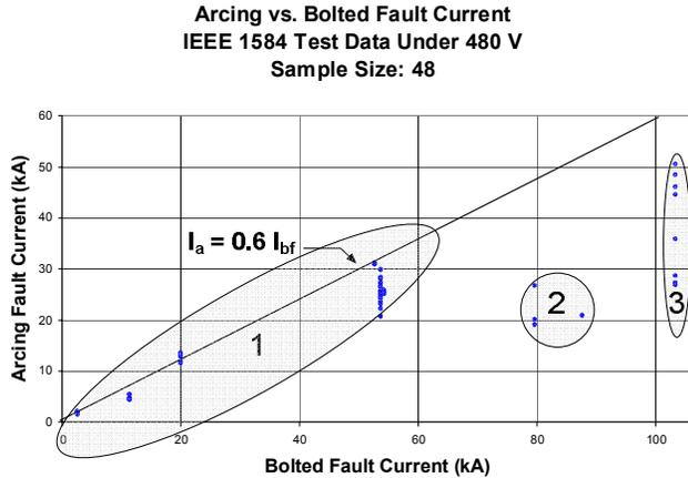
Fig. 2 Scatter-Plot of IEEE 1584 Low Voltage Test Data: 480V and Below
