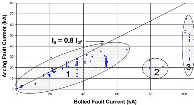
Fig. 5 Scatter-Plot of IEEE 1584 Low Voltage Test Data: 600V and Below
