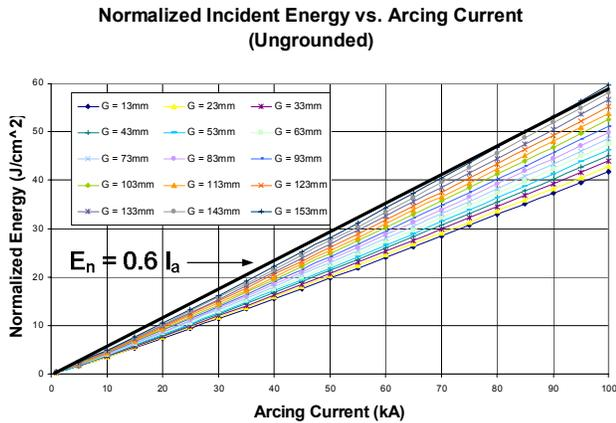
Fig. 9 Sensitivity to Gap between Conductors: Over 1kV
