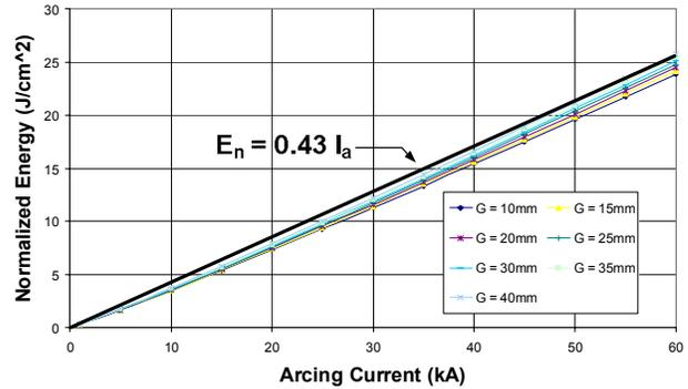
Fig. 3 Sensitivity to Gap between Conductors: 480V and Below
