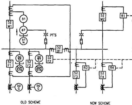
Figure 4 Bus and Feeder Protection
