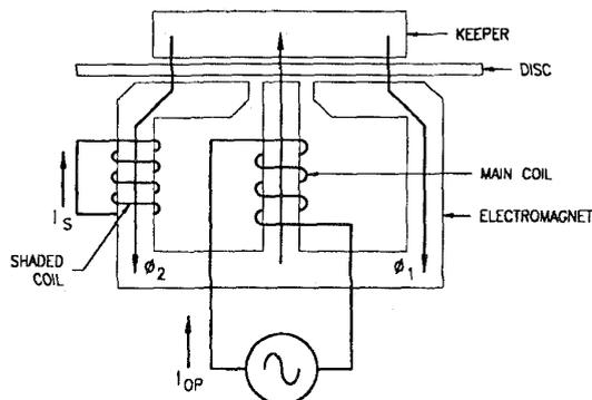
Figure 1 Shaded Pole Electromagnetic Circuit
