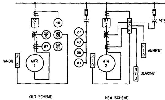
FIGURE 4 MOTOR PROTECTION
