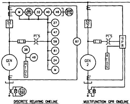
Figure 2 Generator Protection Scheme
